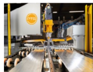
Automated FSW cell for automotive battery trays
