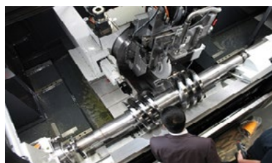
Large screw pump-spindle grinding machine tool
