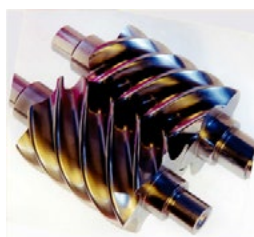
Steel screw-compressor rotors (HVAC)
